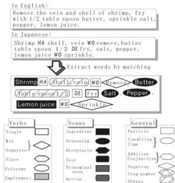
Figure 4.2: Process 1. Extract words by matching with the dictionaries.
