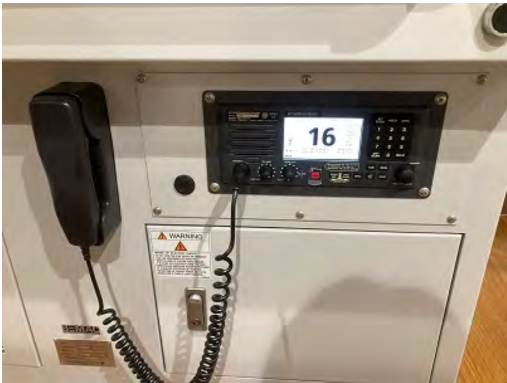
Fig. 6.4: Configuration of Shiphandling Simulator 【International VHF Radio Telephone System】
