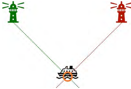
Fig. 2.3: Position acquisition by cross bearing[25]
