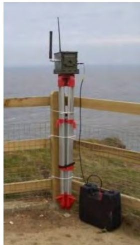
Fig. 4.1: GPS jammer unit installed in Flamborough Head, England [49]
