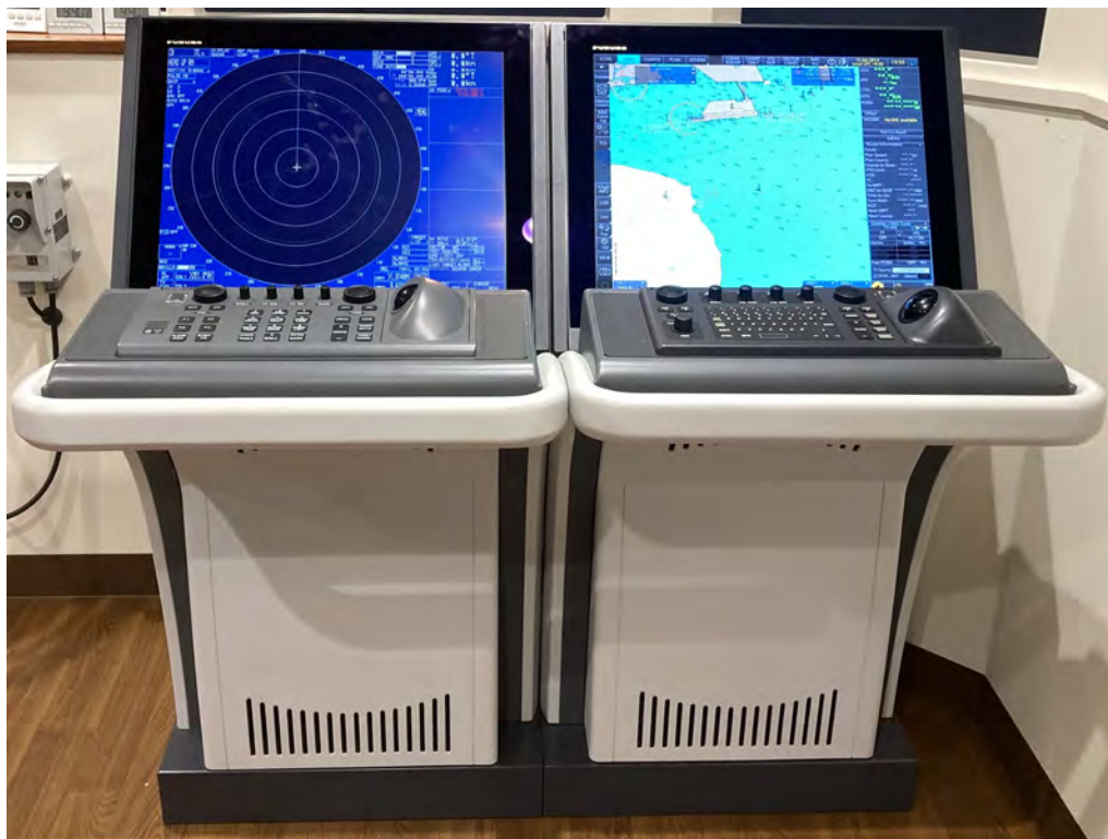
Fig. 6.2: Configuration of Shiphandling Simulator [Marine Radar (Left), ECDIS (Light)]
